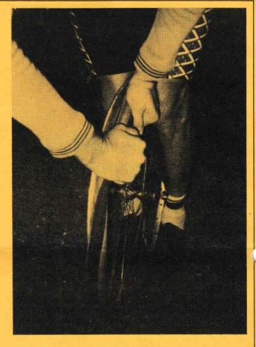
upwards. The reason for this will be revealed in due course. Now you can fish around inside the tyre and remove the punctured tube.
